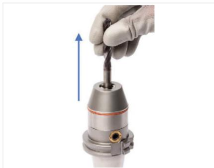
Fig. 6: Remove the tool
