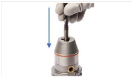
Fig. 3: Inserting tool
