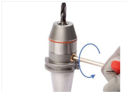
Fig. 5: Loosening pinion
