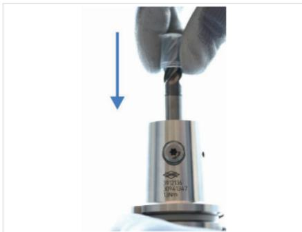
Fig. 3: Inserting tool
