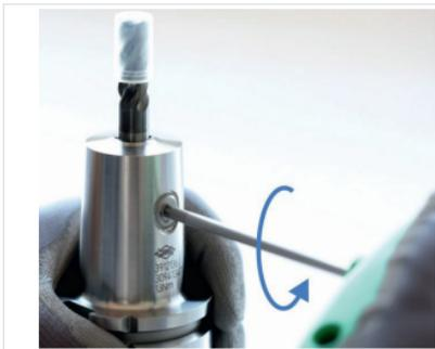
Fig. 6: Loosening clamping screw
