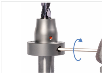
Fig. 11: Tightening clamping screw 2
