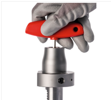
Fig. 8: Adjusting tool length (axial)
