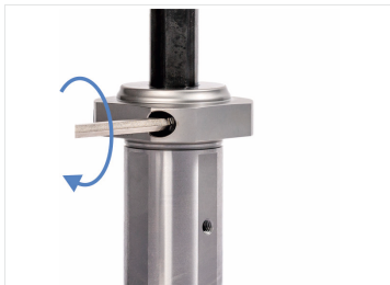
Fig. 21: Tightening clamping screw
