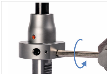
Fig. 18: Loosening locking screw
