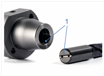
Fig. 7: Cleaning hydraulic chuck and tool
