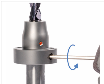
Fig. 12: Loosening clamping screw
