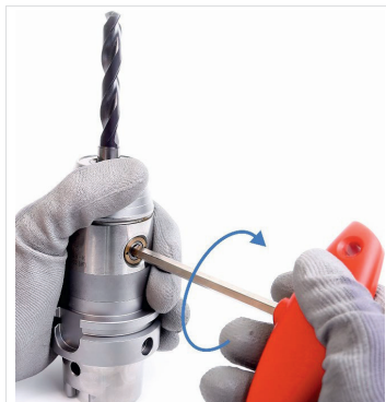
Fig. 6: Clamp the tool
