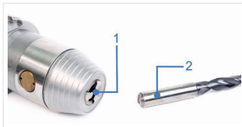
Fig. 4: Cleaning precision drill chuck and tool
