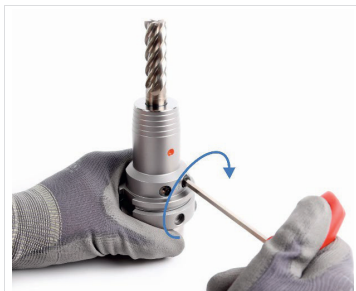
Fig. 10: Clamp the tool
