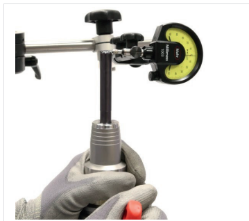
Fig. 17: Adjusting the radial run-out
