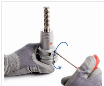
Fig. 13: Loosening clamping screw
