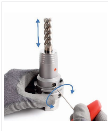
Fig. 11: Adjusting tool length (radial)
