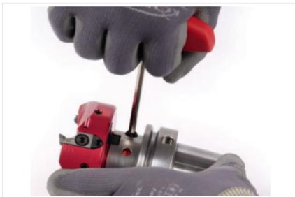
Fig. 9: Loosening clamping screw
