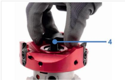
4. Turn the milling cutter clamping screw (4) by hand into the location bore of the hydraulic clamping arbor.
