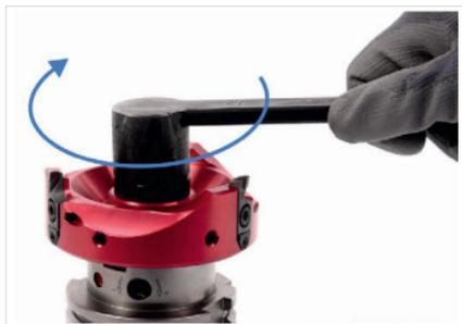
Fig. 7: Tighten the milling cutter clamping screw
