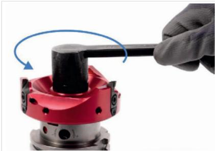
Fig. 8: Loosening the milling cutter clamping screw
