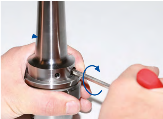
Figure 2: Tighten the clamping screw and observe the minimum revolutions
