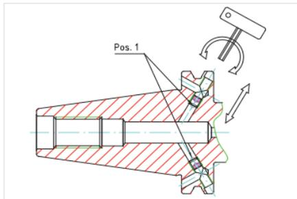
Fig. 14: Normal setting of the coolant supply
