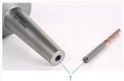
Fig. 8: Cleaning hydraulic chuck and tool
