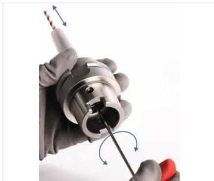
Fig. 10: Adjusting the tool length
