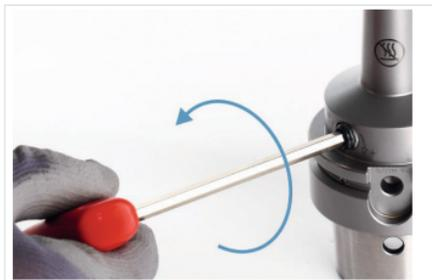
Fig. 12: Loosening clamping screw
