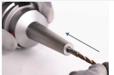
Fig. 9: Inserting tool
