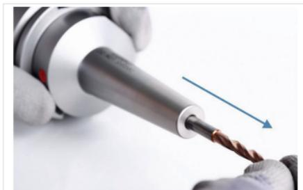
Fig. 13: Removing tool
