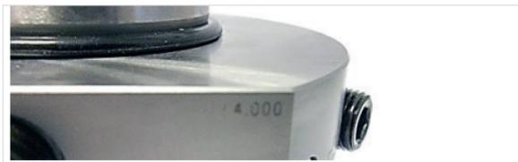
Fig. 5: Marking for checking of the clamping force
