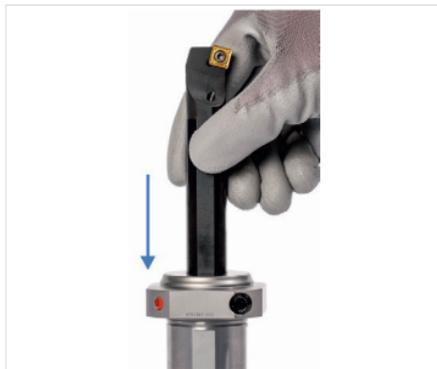
Fig. 19: Inserting tool
