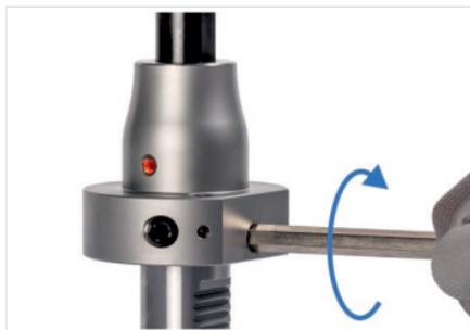
Fig. 15: Tightening locking screw
