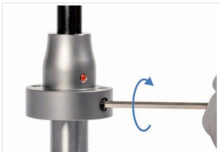
Fig. 16: Tightening clamping screw 2
