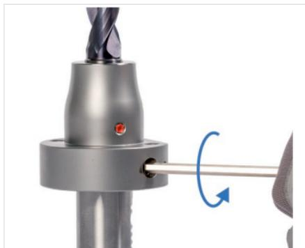
Fig. 12: Loosening clamping screw
