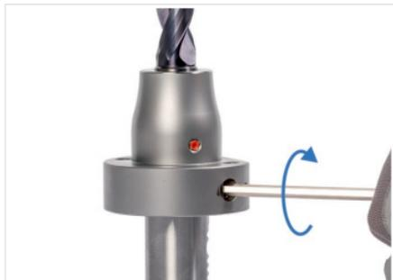
Fig. 11: Tightening clamping screw 2
