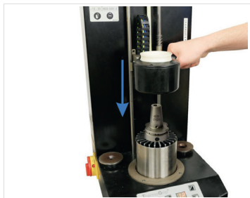
Fig. 7: Heat the shrink chuck with shrink unit
