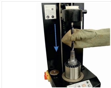
Fig. 8: Insert tool into the location bore
