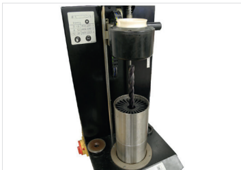
Fig. 9: Cool the shrink chuck with tool.
