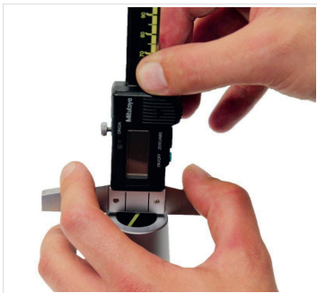
Fig. 6: Set shrink chuck to tool length
