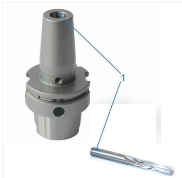
Fig. 5: Clean the shrink chuck and tool
