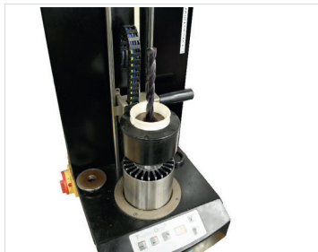
Fig. 10: Heat the shrink chuck with tool
